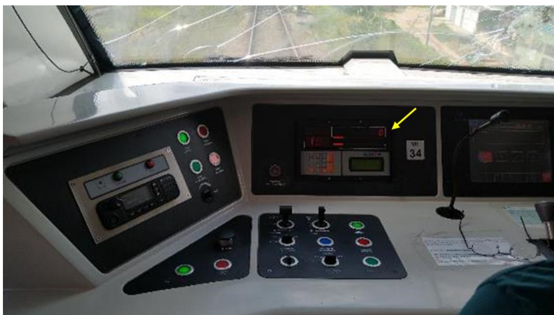
Foto 8-20: Console ATC de Bordo Alstom – TUE CAF
