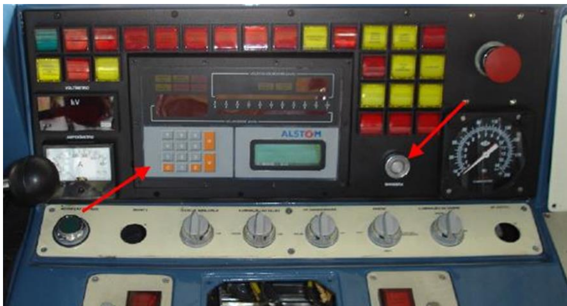
Foto 8-21: Console ATC de Bordo Alstom – TUE CISM
